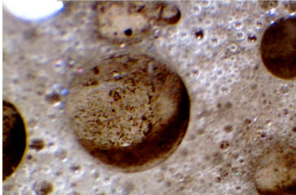
**Micrograph of a nano-iron emulsion dispersed in water Mag= 1000X.
